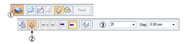
• Click Finish to complete the extrusion. The sketch is still displayed with the new protrusion.
