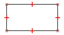
You can also use the Connect command to connect the endpoint of an element to any point on another element, not necessarily an endpoint or keypoint. This is called a point-on-element connection, and the symbol resembles an X. For example, the endpoint of the top horizontal line on the right side of the profile is connected to the vertical line, but not at an endpoint.
