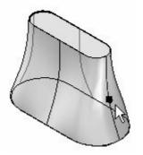
Click the Relative/Absolute Position button . Absolute uses the actual X-Y-Z coordinates for positioning. Relative uses a delta distance for positioning. Use relative positioning.
